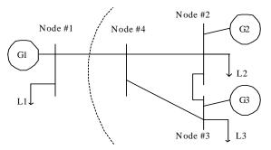
Figure 1. A 4-node DC network with four branches
